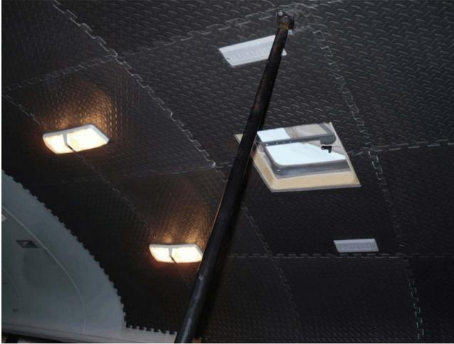
This photo was taken from the front step of the bus, looking in. It shows the vent installed, and several courses of tiles glued in place. You will also see four lights in place. Two are the original Carpenter Bus lights. They run off of the main battery. The others, which are lit, I installed. They run off of auxiliary power, or shore power and have switches on each light. These too were salvaged from the RV in Tennessee.
