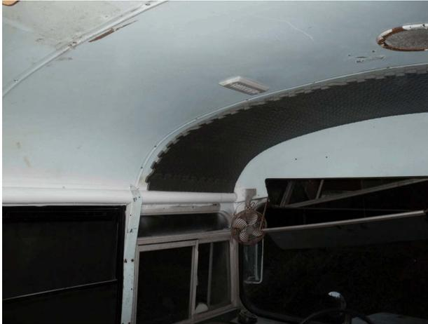
And here is the final piece in place for the first course of tile. I had to take a break from gluing tile at this point, for I needed to install a ceiling vent. I had salvaged a vent from the RV in Tennessee. There was previously a small round vent in the ceiling, which can be seen in these pictures, but it was inadequate, and had been painted completely shut up on the roof. I needed to cut a hole, and install the new vent, before putting more ceiling tiles up.
