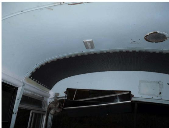
Pictured above is the first row of tile all the way to the opposite side. All that is left is the final edge piece to dress out the boundary between the wall and
