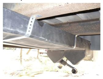
Gray Water and Black Water Holding Tanks Strapped to Undercarriage
