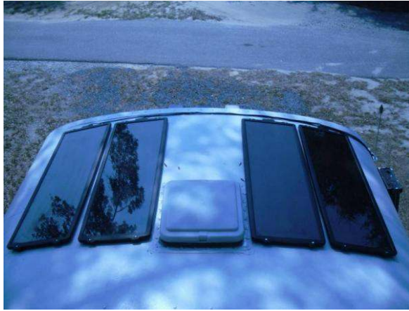
Solar Panels on Roof of The Dreamer
